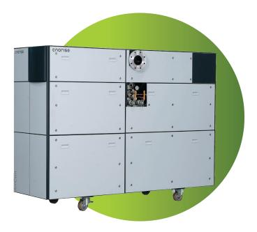
Combustion air pressure, temperature and humidity have a significant influence on an internal combustion engine's power output and exhaust emissions. To gain a good reproducibility of measuring results, and with this an increased test cell utilization, these conditions must be kept constant within narrow limits.
